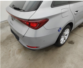
Bumper Rear // Painting-scratch + dent
