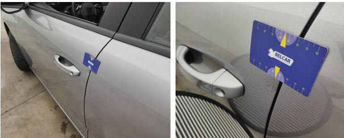
Door Front Left // Repair & Painting-scratch + dent
