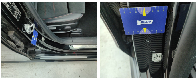
Rocker Panel Right // Smart Repair Medium-scratch + dent
