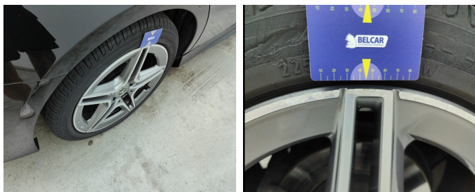
Tyre Rear Right // Replace-tear
