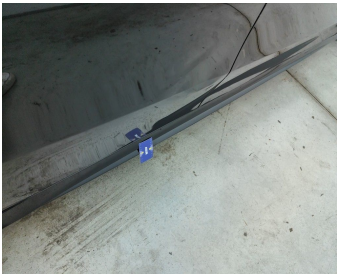
Rocker Panel Right / Cover Not Painted / Replace-dent
