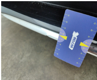
Rocker Panel Right / Cover Not Painted / Replace-dent
