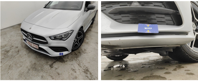
Bumper Front / Trim Left / Replace-scratch
