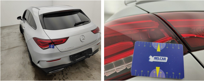
Light / Rear left / Replace-scratch
