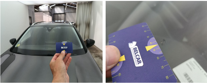
Windshield // Replace-glass damage
