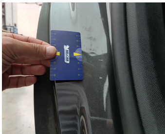
Rocker Panel Right // Smart Repair Medium-scratch
