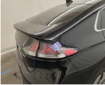
Light / Rear Right / Replace-cracked
