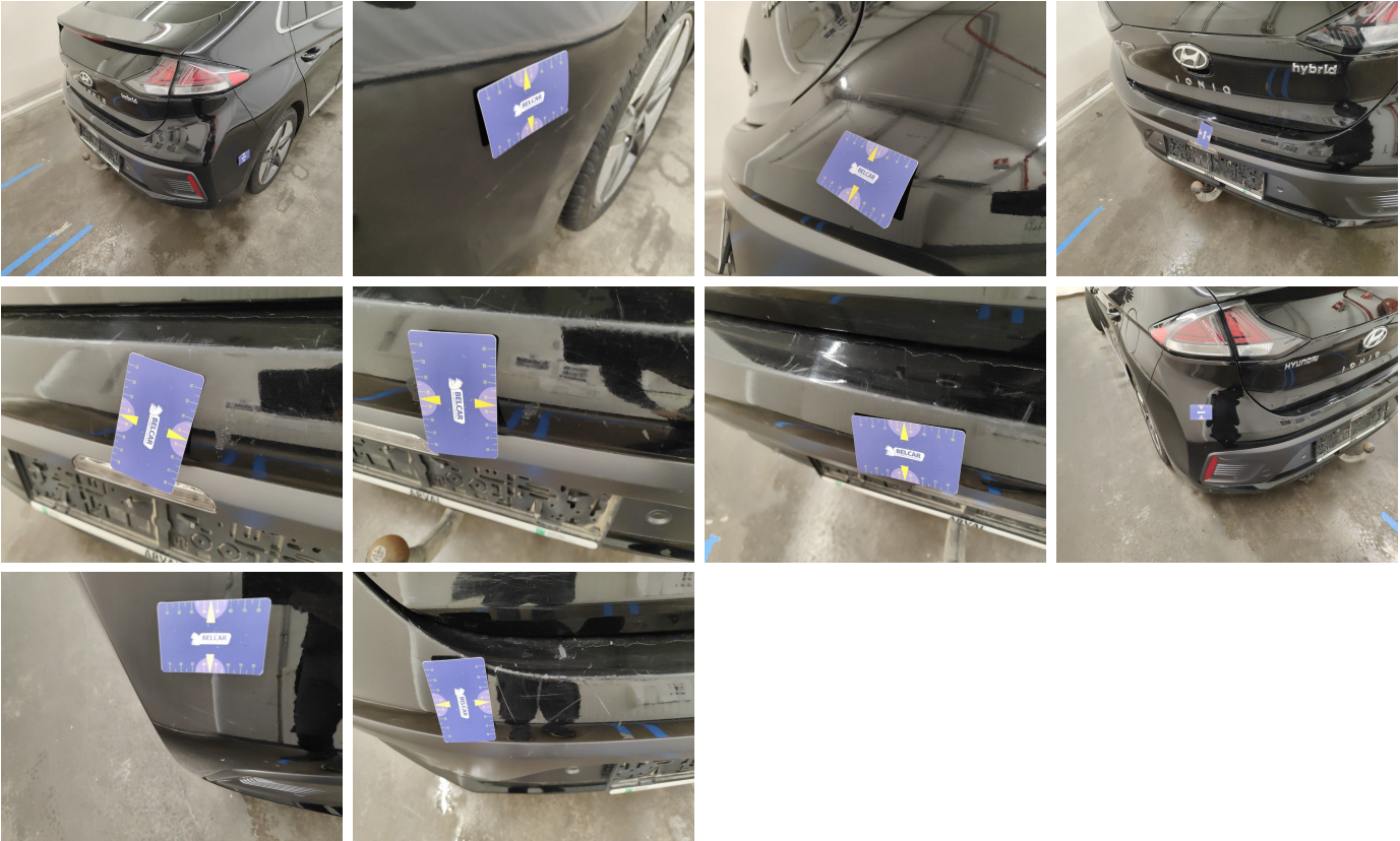
Bumper Rear // Painting-scratch
