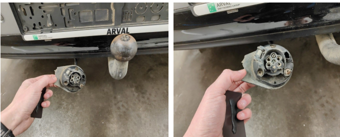
Towing Cover Rear // Replace-cracked
