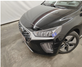
Headlight / Front left / Replace-scratch
