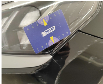
Headlight / Front left / Replace-scratch
