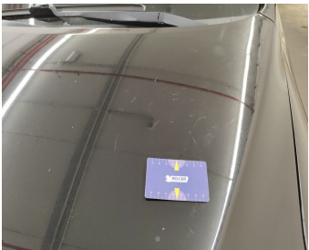
Front Bonnet // Painting-scratch + dent
