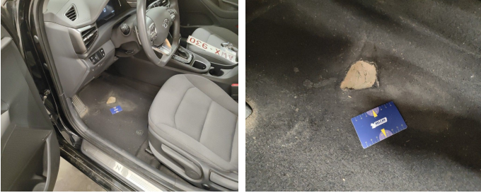
Interior / Floor Covering / Replace-hole
