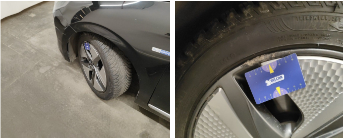
Damage within Renta-norm-scratch
