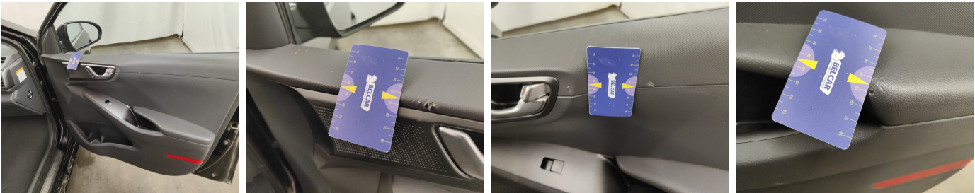
Front Right Door Interior Coating // Replace Completely- tear
