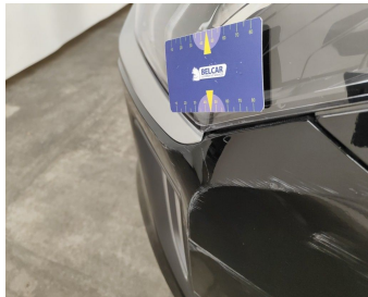
Headlight / Front left / Replace-scratch
