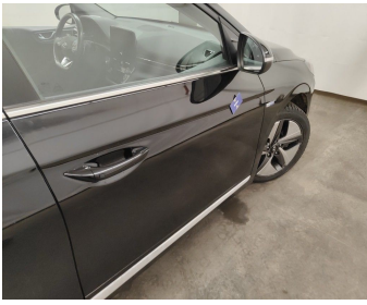
Door Front Right // Painting-bad repair
