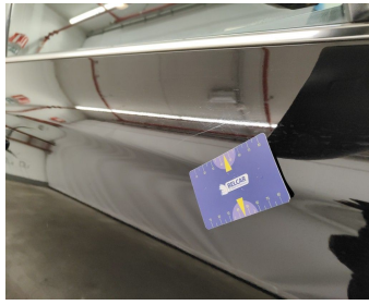
Door Front Right // Painting-bad repair
