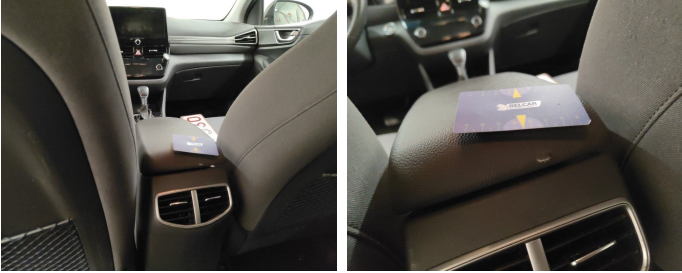
Central Console / Cover Armrest / Replace Cover Armrest-tear
