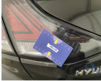
Light / Rear Left On Rear Bonnet / Replace-scratch
