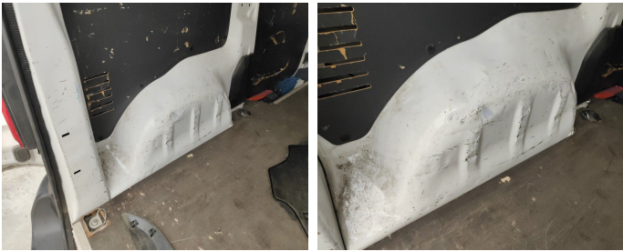
Trunk Compartment / Side Cover Left / Replace-scratch + dent
