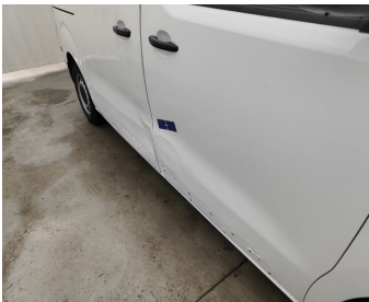
Door Front Right // Repair & Painting-scratch + dent
