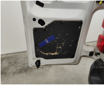
Trunk Lid Interior Coating / MDF Rear Left / Replace- cracked
