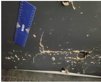
Trunk Lid Interior Coating / MDF Side Door Right / Replace-cracked
