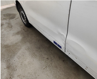
Rocker Panel Right // Repair & Painting-scratch + dent
