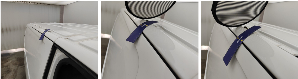
Roof // Repair & Painting-scratch + dent
