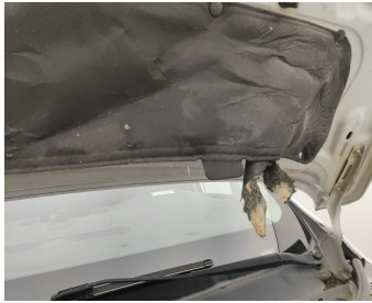
Front Bonnet / Insulation / Replace-tear
