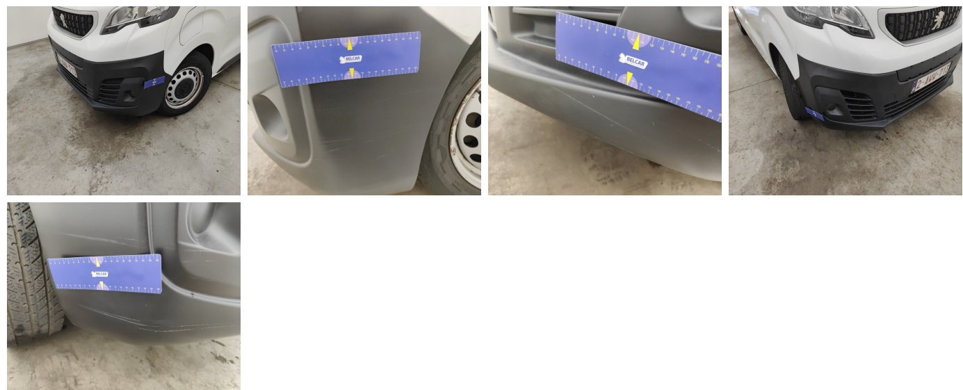
Bumper Front / Lower Cover Not Painted / Replace-scratch
