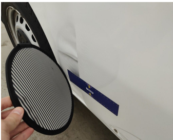
Door Rear Right // Repair & Painting-scratch + dent
