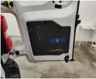
Trunk Lid Interior Coating / MDF Rear Right / Replace- cracked
