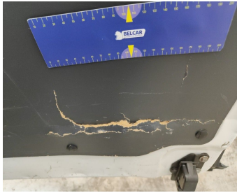
Trunk Lid Interior Coating / MDF Rear Right / Replace- cracked
