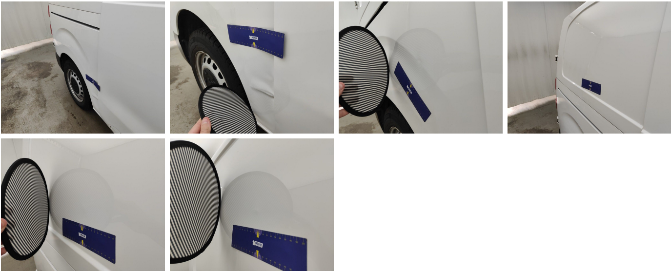
Wing Rear Right // Repair & Painting-scratch + dent
