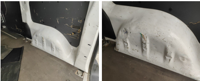
Trunk Compartment / Side Cover Right / Replace-scratch + dent
