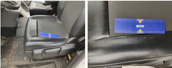
Seat Front Left / Bottom Coating / Replace-worn
