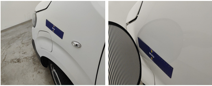
Wing Front Left // Repair & Painting-scratch + dent
