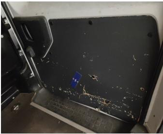
Trunk Lid Interior Coating / MDF Side Door Right / Replace-cracked
