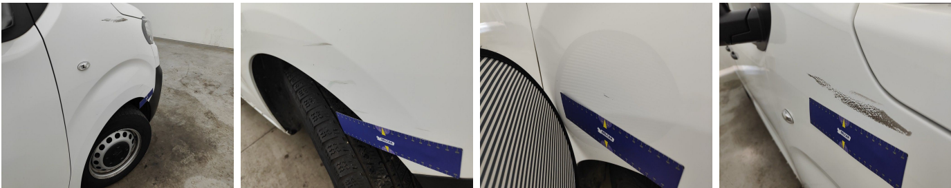
Wing Front right // Repair & Painting-scratch + dent
