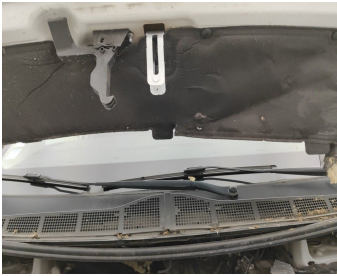
Front Bonnet / Insulation / Replace-tear
