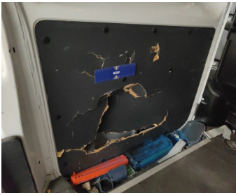
Trunk Lid Interior Coating / MDF Side Door Left / Replace-cracked
