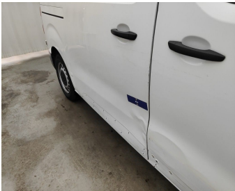
Rocker Panel Right // Repair & Painting-scratch + dent
