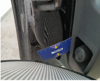
Door Front Left // Repair & Painting-dent
