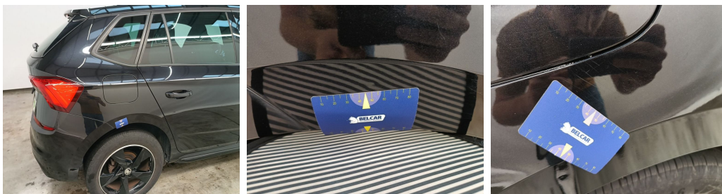
Wing Rear Right // Repair & Painting-dent
