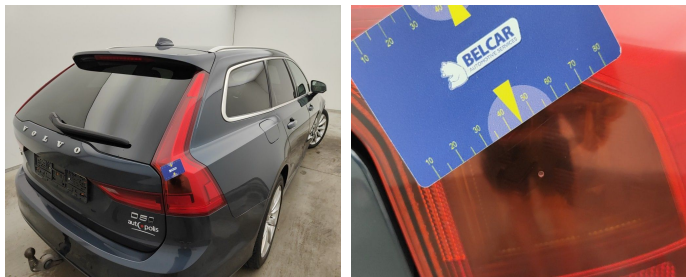
Light / Rear Right / Replace-scratch
