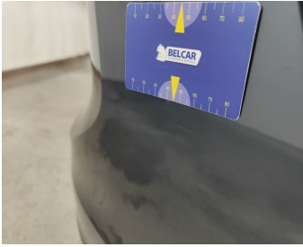
Bumper Rear // Painting-bad repair
