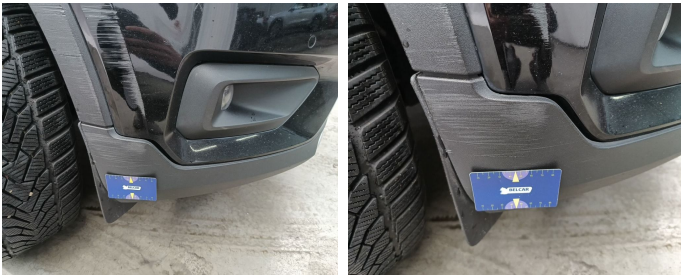
Bumper Front / Lower Cover Not Painted / Replace-scratch
