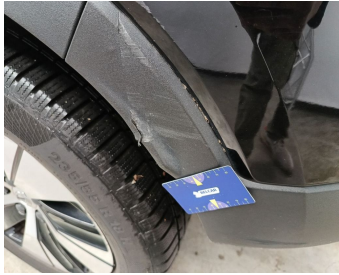
Bumper Rear / Lower Cover Not Painted / Replace-cracked
