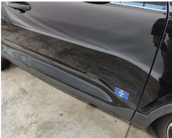
Door Front Right // Repair & Painting-scratch + dent
