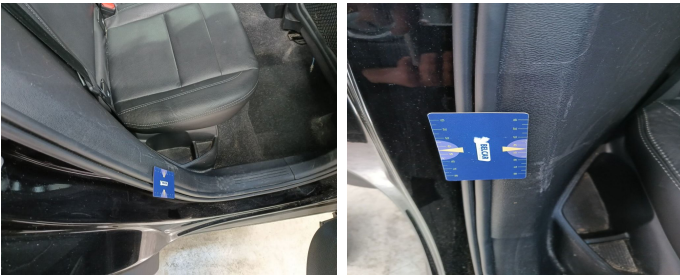
Interior / Side Cover rear Seat / Replace-scratch
