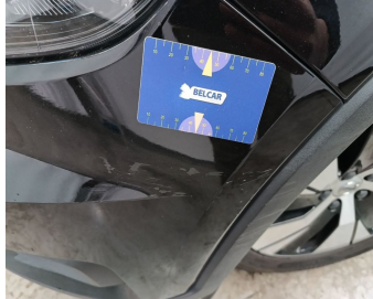
Bumper Front / Lower Cover Not Painted / Replace-scratch
