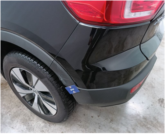
Bumper Rear / Lower Cover Not Painted / Replace-cracked
