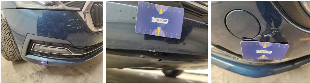
Bumper Front // Replace & Painting-cracked
