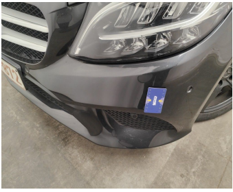
Bumper Front // Painting-bad repair
