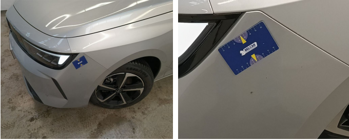
Bumper Front // Painting-stone chipping
