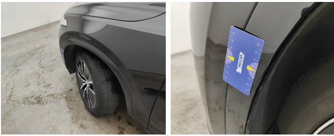
Wing Front Left / Trim / Replace-scratch
