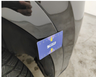
Wing Front right / Trim / Replace-scratch
