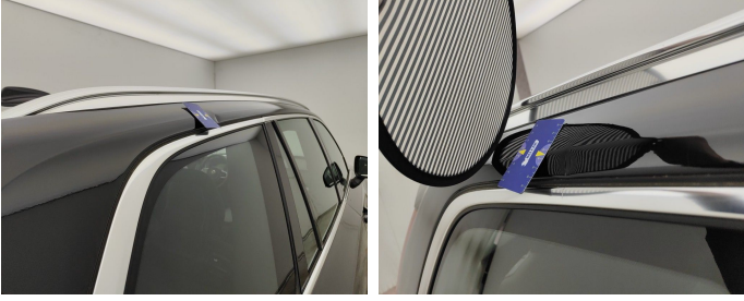
Roof // Smart Repair Medium-scratch + dent
