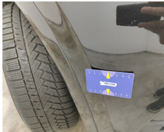
Wing Front right / Trim / Replace-scratch
