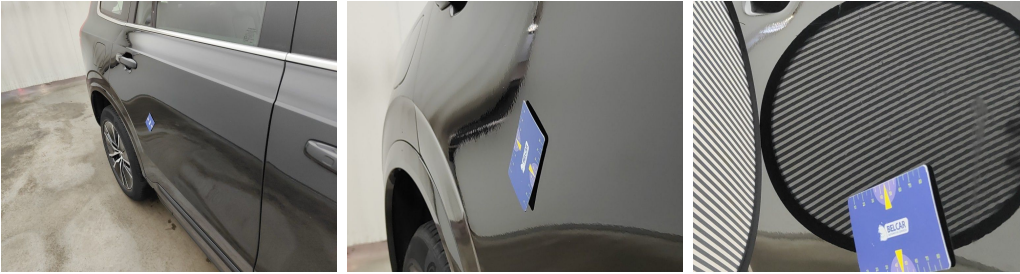
Door Rear Right // Painting-bad repair
