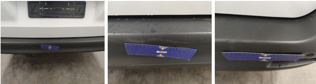
Bumper Rear / Lower Cover Not Painted / Replace-scratch
