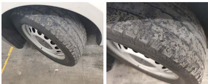
Tyre Front Left // Replace-worn
