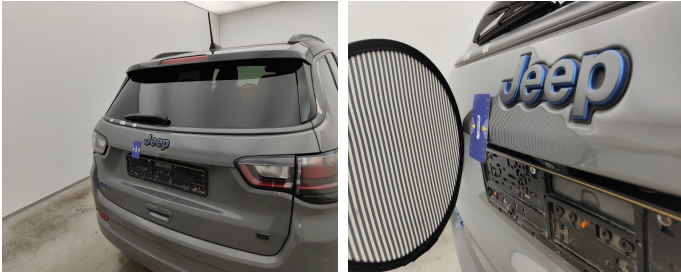
Rear Bonnet // Painting-bad repair
