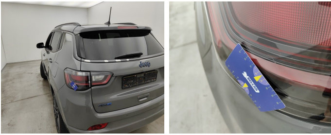
Light / Rear left / Replace-scratch
