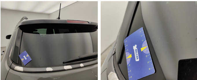
Rear Bonnet / Rear Window / Replace-scratch
