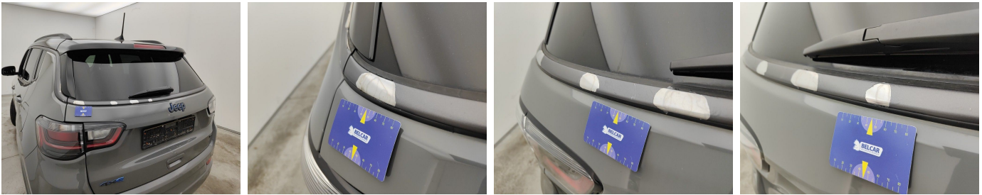
Rear Bonnet / Trim / Replace-bad repair
