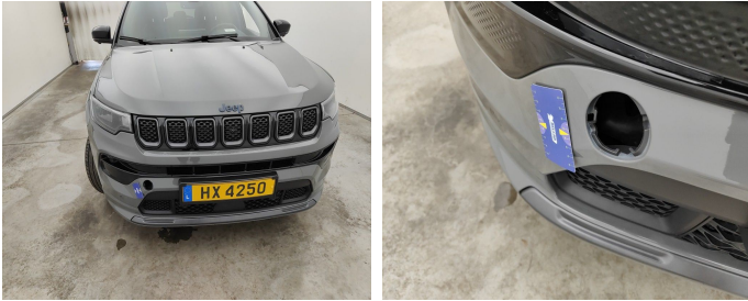
Front / Towing Cover / Replace-missing
