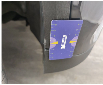
Wing Front right / Trim / Replace-scratch
