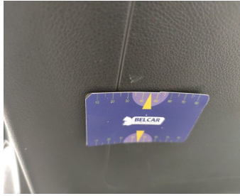
Rocker Panel Right // Smart Repair Medium-scratch
