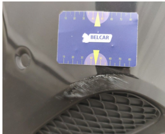
Bumper Front // Smart Repair Medium-scratch
