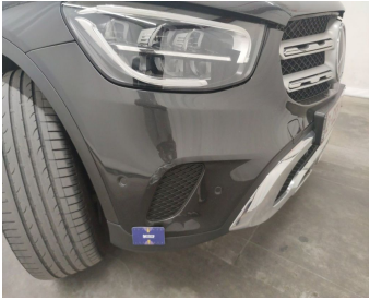
Bumper Front / Lower Cover Not Painted / Replace-scratch
