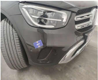
Bumper Front // Smart Repair Medium-scratch
