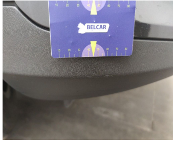
Bumper Front / Lower Cover Not Painted / Replace-scratch
