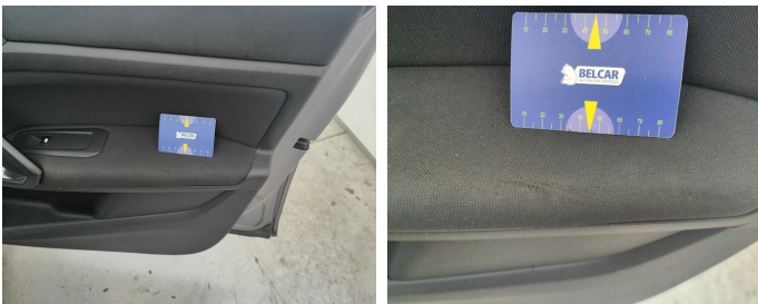
Front Right Door Interior Coating // Repair-worn
