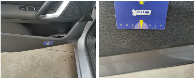
Front Left Door Interior Coating // Repair-scratch
