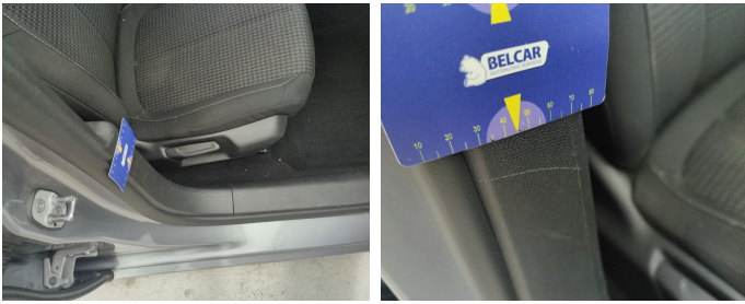
Interior / A Pillar Lower Cover / Replace-scratch
