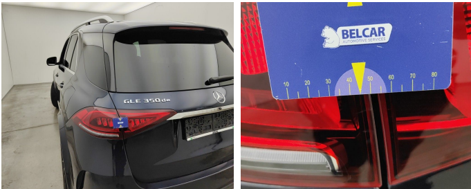
Light / Rear left / Replace-scratch
