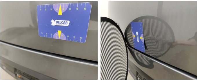
Rear Bonnet // Repair & Painting-scratch + dent
