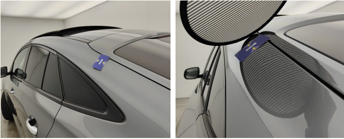
Roof // Smart Repair Medium-dent
