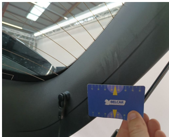
Trunk Lid Interior Coating / Complete Panel / Replace-scratch + dent
