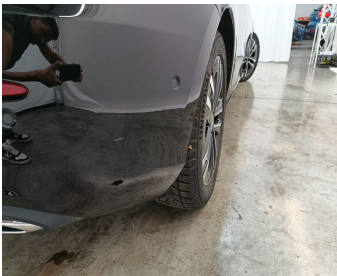
Bumper Rear // Repair & Painting-scratch + dent
