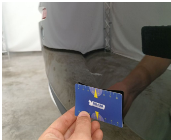
Bumper Rear // Repair & Painting-scratch + dent
