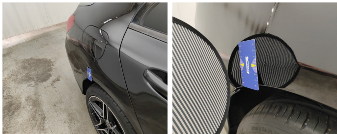
Wing Rear Right // Repair & Painting-scratch + dent
