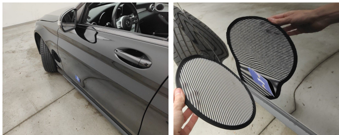
Door Front Left // Painting-bad repair
