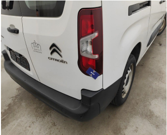
Light / Rear Right / Replace-scratch
