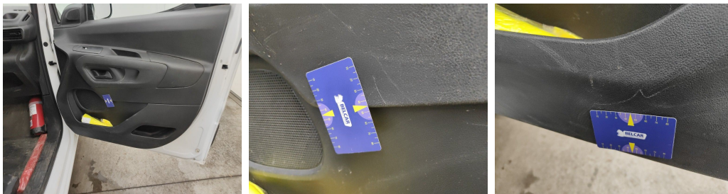
Front Right Door Interior Coating // Replace Completely-scratch
