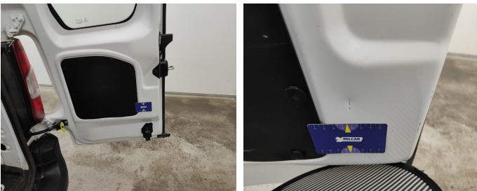
Rear Loading Door Right // Repair & Painting-scratch + dent
