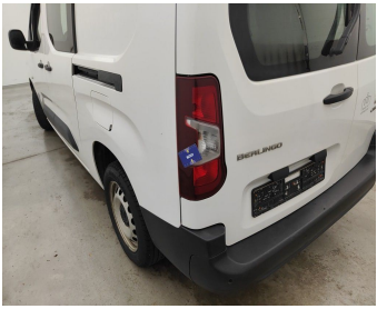
Light / Rear left / Replace-scratch
