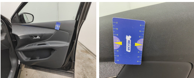
Front Right Door Interior Coating // Replace Completely-scratch
