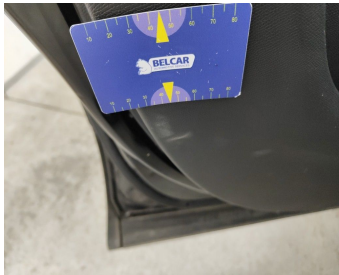
Rear Left Door Interior Coating // Replace Completely-scratch + dent
