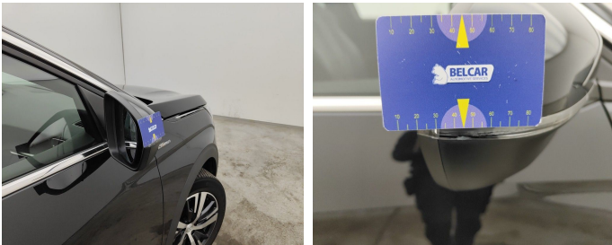
Side View Mirror Right / Direction Indicator / Replace-scratch
