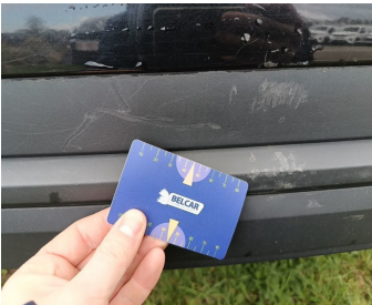
Bumper Rear / Lower Cover Not Painted / Replace-scratch
