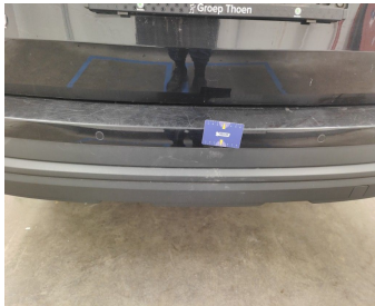
Bumper Rear / Lower Cover Not Painted / Replace-scratch
