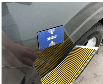
Wing Rear Right // Smart Repair Small-dent
