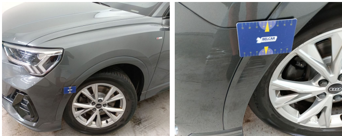
Wing Front Left / Trim / Replace-scratch
