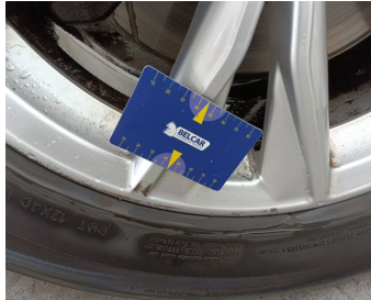
Wheel Alloy Front Left // Repair-scratch
