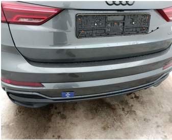
Bumper Rear / Lower Cover Not Painted / Replace-scratch
