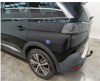
Wing Rear Left // Repair & Painting-scratch + dent
