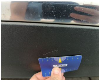
Door Front Right / Trim / Replace-scratch
