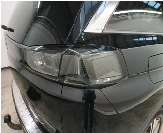
Light / Rear Right / Replace-scratch
