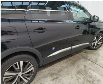
Rocker Panel Right // Smart Repair Medium-scratch + dent
