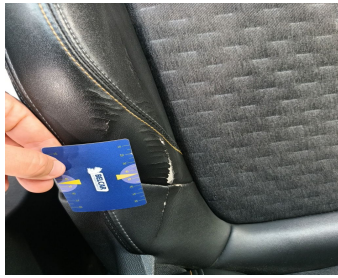
Seat Front Left / Bottom Coating / Replace-worn
