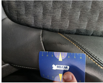
Seat Front Right / Bottom Coating / Replace-worn
