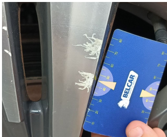
Wheel Two Tone Rear Right // Repair-Chemical reaction
