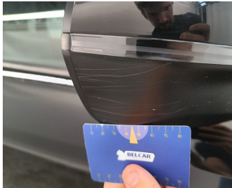
Side View Mirror Right // Plastic Repair-scratch
