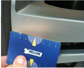
Wheel Two Tone Rear Left // Repair-scratch
