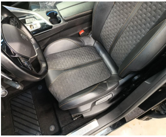
Seat Front Left / Bottom Coating / Replace-worn
