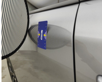
Door Rear Right // Smart Repair Small-dent
