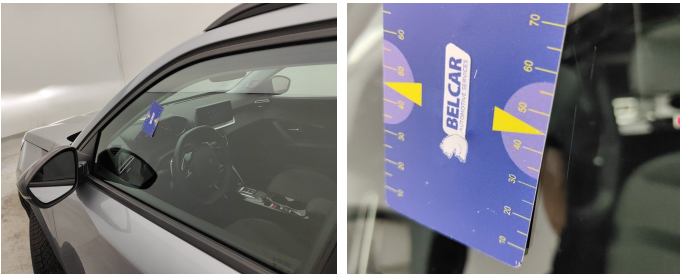
Door Front Left / Window / Replace-scratch
