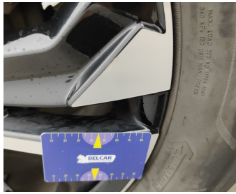
Wheel Two Tone Rear Left // Repair-scratch
