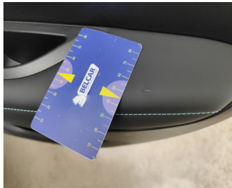
Rear Right Door Interior Coating // Repair-scratch
