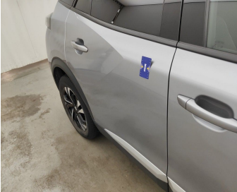
Door Rear Right // Smart Repair Small-dent
