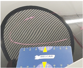
Roof // Smart Repair Medium-dent
