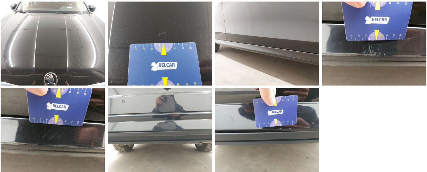
Damage within Renta-norm-Chemical reaction
