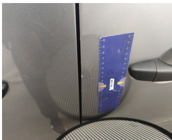
Door Front Right // Repair & Painting-scratch + dent
