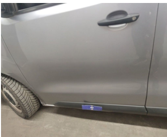
Door Front Right // Repair & Painting-scratch + dent
