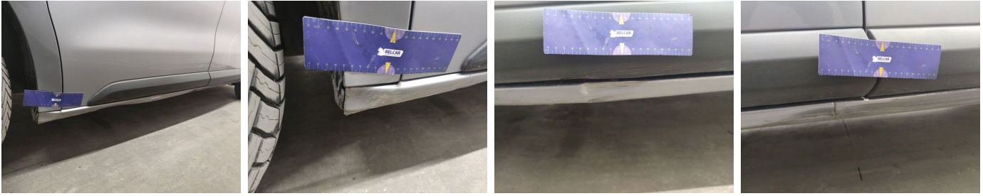
Rocker Panel Left // Repair & Painting-scratch + dent
