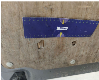
Trunk Lid Interior Coating / MDF Rear Left / Replace-hole
