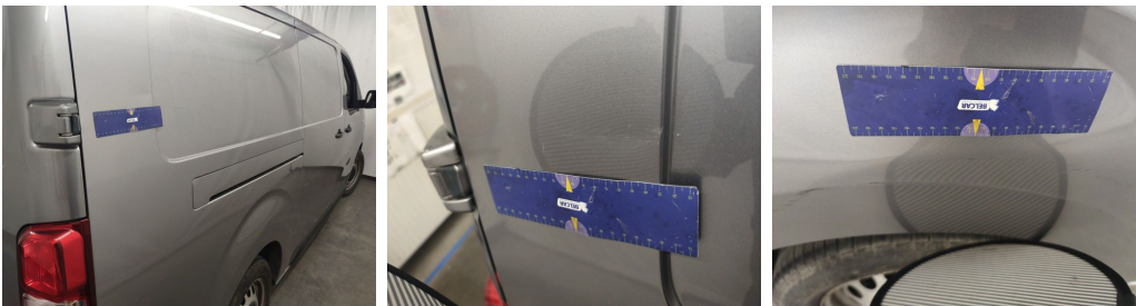
Wing Rear Right // Repair & Painting-scratch + dent
