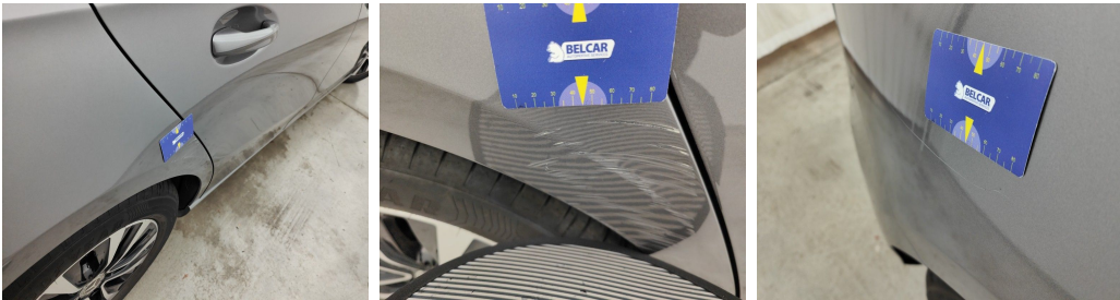
Wing Rear Right // Repair & Painting-scratch + dent
