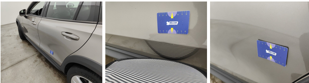
Door Rear Left // Smart Repair Medium-scratch + dent
