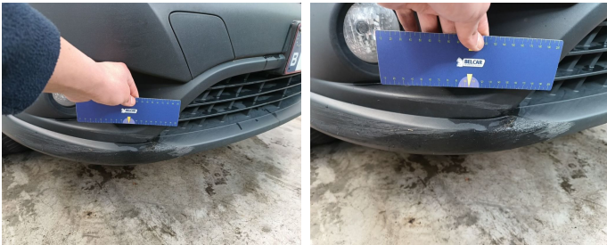
Bumper Front // Replace without painting-scratch + dent
