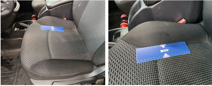
Seat Front Left / Bottom Coating / Replace-tear
