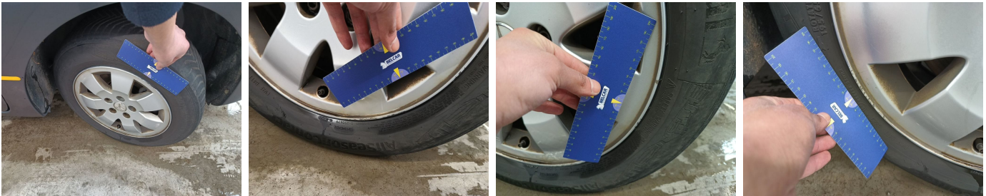
Wheel Alloy Front Right // Repair-scratch
