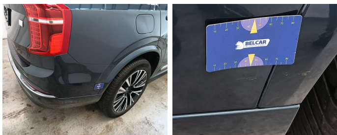
Bumper Rear // Smart Repair Medium-scratch
