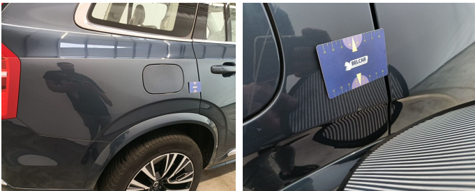
Wing Rear Right // Repair & Painting-scratch + dent
