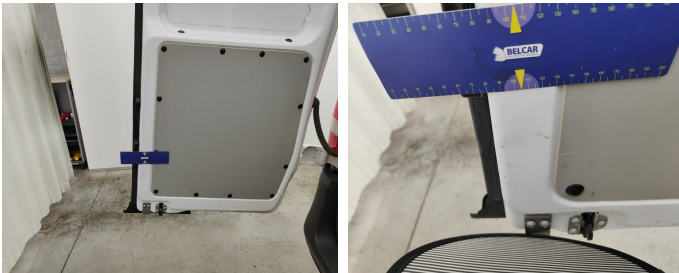
Rear Loading Door Left // Smart Repair Medium-dent
