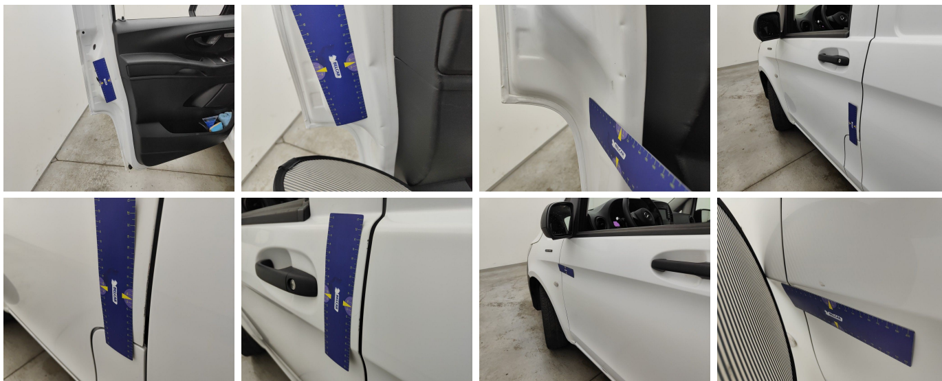
Door Front Left // Repair & Painting-scratch + dent
