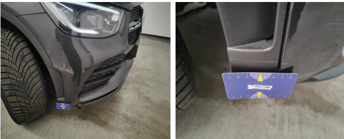
Bumper Front / Trim Right / Replace-scratch
