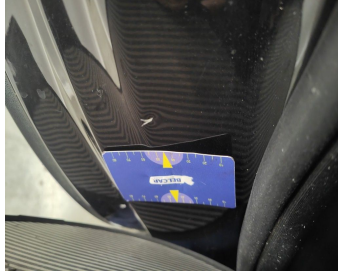
Rocker Panel Right // Smart Repair Medium-scratch + dent
