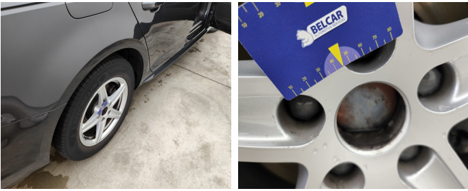
Wheel Rear Right / Hub Cover with Logo / Replace-missing
