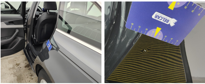
Wing Rear Left // Smart Repair Large-scratch + dent
