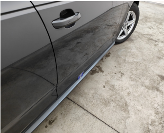
Rocker Panel Right / Cover Not Painted / Replace-scratch
