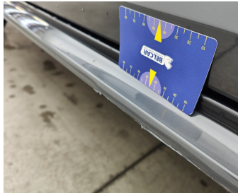
Rocker Panel Right / Cover Not Painted / Replace-scratch
