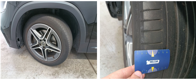
Tyre Front Left // Replace-worn
