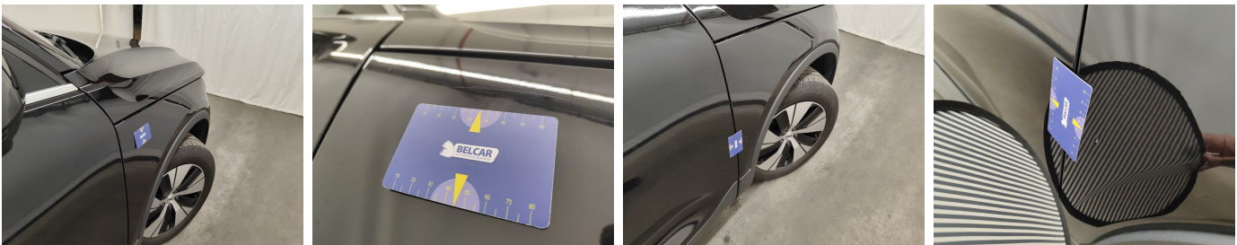
Wing Front right // Repair & Painting-scratch + dent
