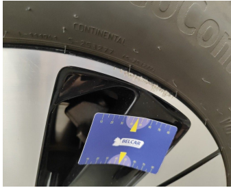
Wheel Two Tone Front Right // Repair-scratch
