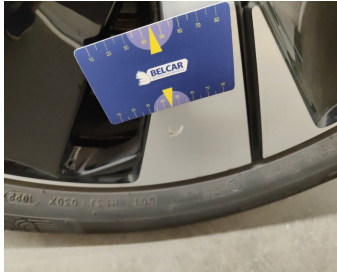
Wheel Two Tone Rear Left // Repair-scratch
