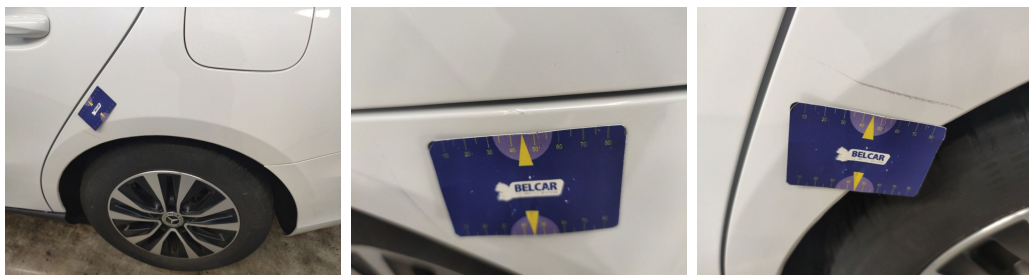
Wing Rear Left // Painting-bad repair
