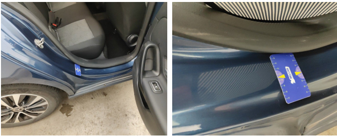
Rocker Panel Right // Smart Repair Medium-dent
