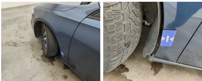
Wing Front Left / Inner Fender / Replace-bad position
