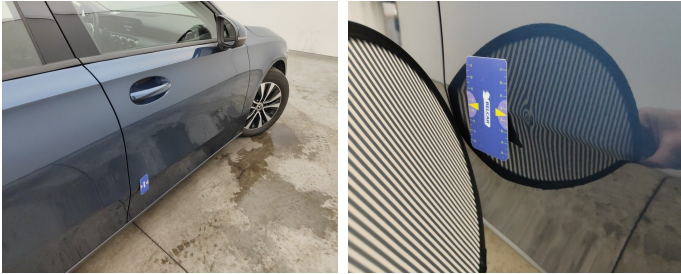
Door Front Right // Repair & Painting-dent
