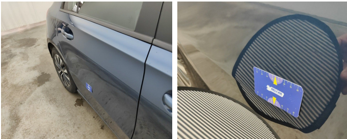
Door Rear Right // Repair & Painting-scratch + dent
