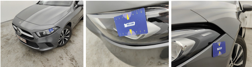
Headlight / Front left / Replace-bad position
