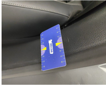
Interior / Side Cover rear Seat / Replace-scratch
