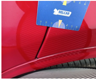
Wing Rear Left // Repair & Painting-scratch + dent
