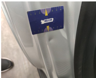
Rocker Panel Right // Smart Repair Medium-dent
