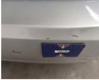
Bumper Rear // Repair & Painting-scratch + dent
