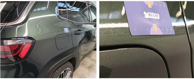
Wing Rear Right // Painting-bad repair
