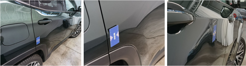
Door Rear Right // Painting-bad repair
