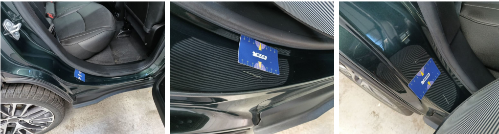
Rocker Panel Right // Smart Repair Medium-scratch + dent
