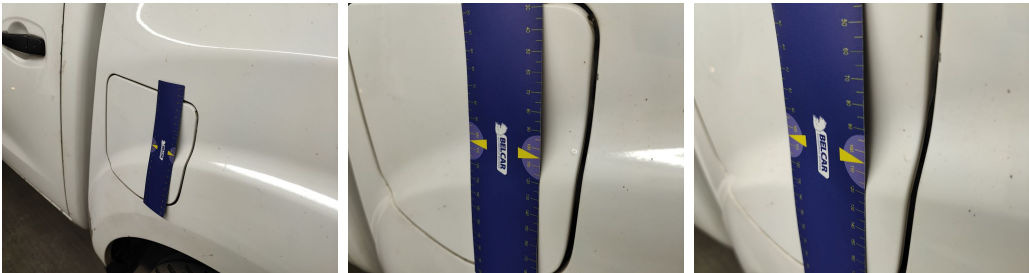
Back Side // Repair & Painting-bad repair
