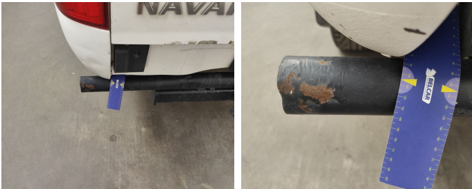
Bumper Rear / Lower Cover Not Painted / Replace-rust
