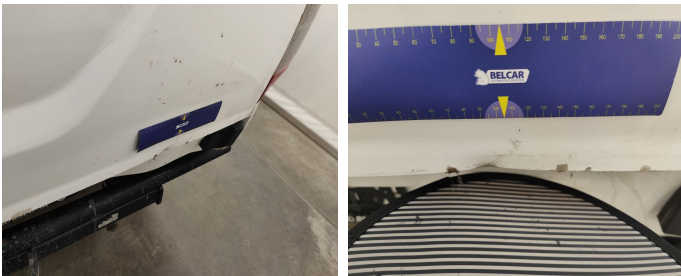
Bumper Rear // Repair & Painting-dent
