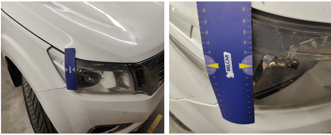
Light / Front Right / Replace-scratch
