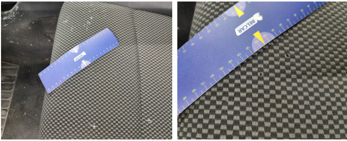
Seat Front Left / Bottom Coating / Replace-Incinerated
