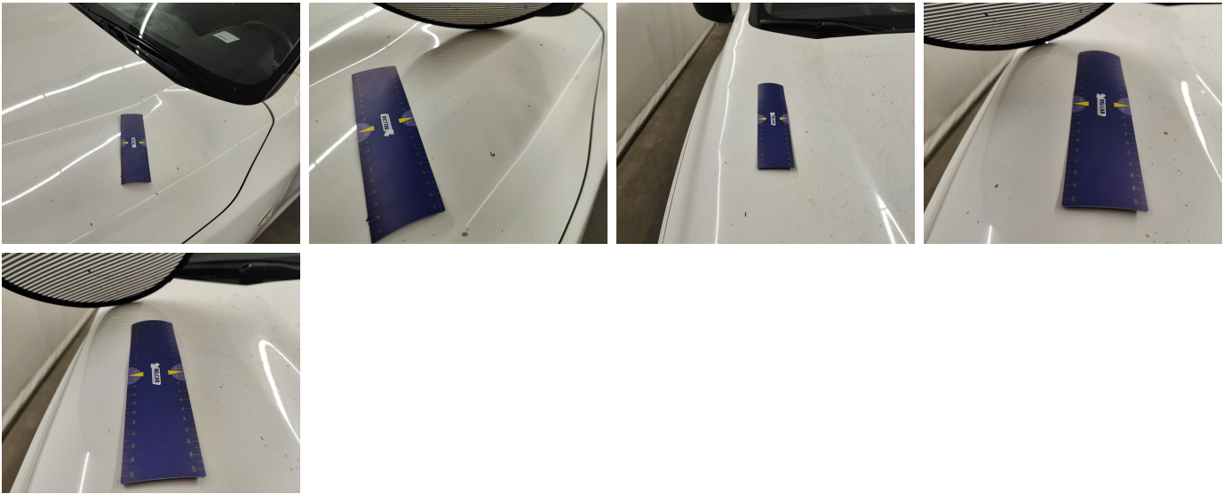
Front Bonnet // Repair & Painting-dent
