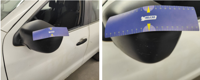
Side View Mirror Left / Shell / Replace Painted-scratch
