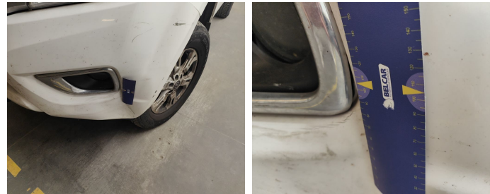
Bumper Front / Trim Left / Replace-bad position
