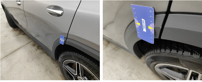
Door Rear Left / Trim / Replace-scratch
