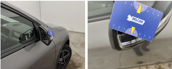
Side View Mirror Right / Direction Indicator / Replace-scratch
