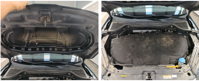
Front Bonnet / Insulation / Replace-bad position
