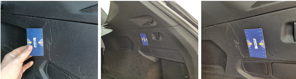
Trunk Compartment / Side Cover Right / Replace-scratch
