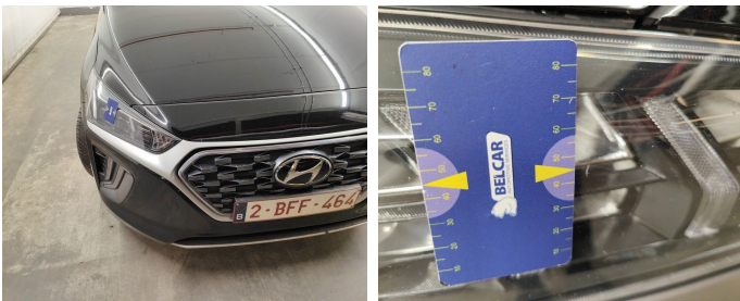
Light / Front Right / Replace-scratch
